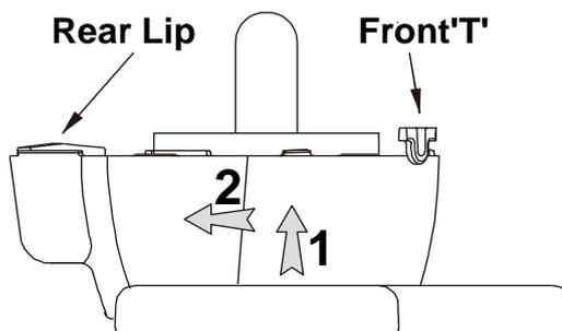
Loosen the thumb-screw at the front of the lamp holder module by about 5mm. Holding the lamp holder module by the Handle, slide it forward until both the rear lip and the front 'T' of the lamp holder module clear their home positions. Reverse this action to replace the lamp holder and then tighten the thumb-screw to lock the lamp holder module into position.
