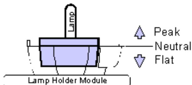
First level the cup with the edge of the module by adjusting the three levelling screws. Then set to the correct height as detailed above.
