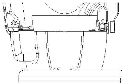
Familiarise yourself with the way the lens tube can be rotated by loosening the lens tube locking clamp and turning the tube. Note how the colour frames are locked into the front of the lens tube with the colour frame locking clip and plunger.
