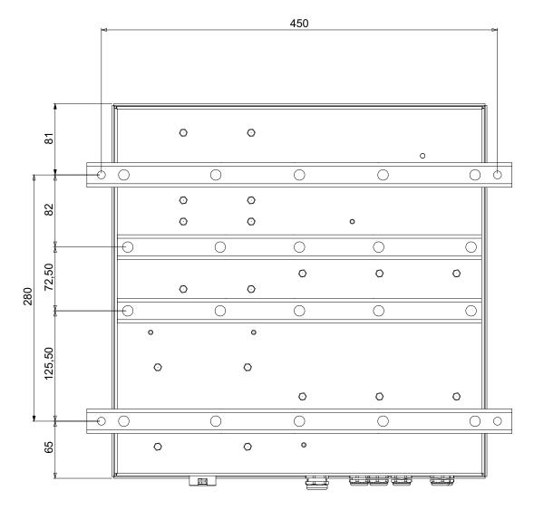
Figure 4: Mounting hole spacing (in mm)
