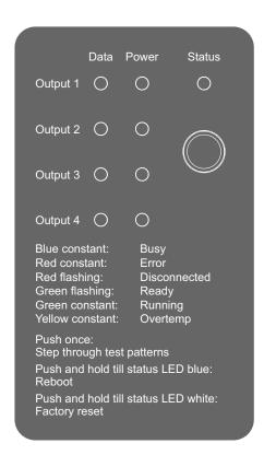
Figure 7: Status LEDs and control button
