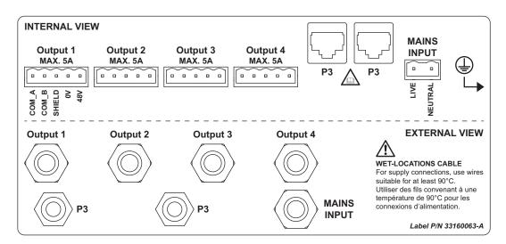
Figure 5: Power and data connections, external and internal views
