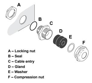
Figure 6: Cable gland assembly
