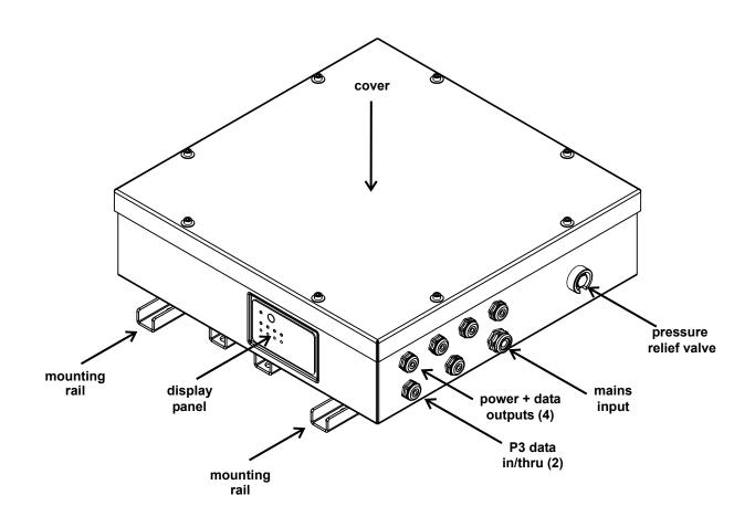
Figure 1: Parts identification
