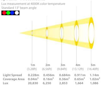
**Spread (m):** The spread is the width of the light when it hits the flat surface. **Coverage Area (m<sup>2</sup>):** The coverage area is the size of the circular area that the light illuminates on the flat surface.
